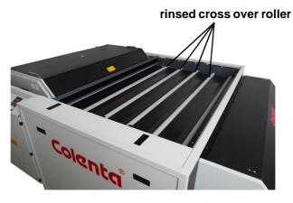
Water rinsed cross over rollers are in place in order to minimize the chemical carry over from one tank to the next as well to keep the cross over section clean and free from any chemical deposits.
