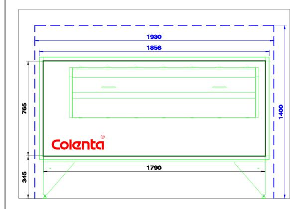
In case the thickness of the wall is more than 2cm, a panel has to be installed this to keep the cover lid of the processor in position - as shown below:
