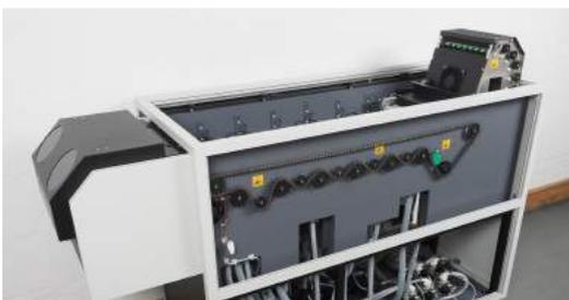
All Colenta Film processors support a maintenance free and reliable chain drive system to drive the wet racks and dryer module.
