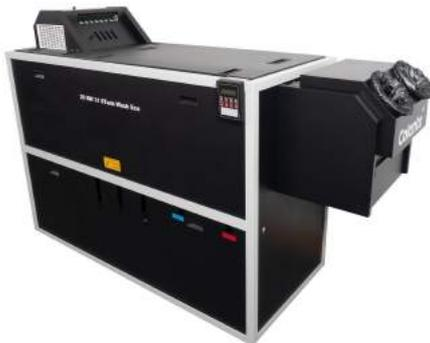
Our 20 B&W models provide an ideal automated and flexible system to develop film in fast time at the processing parameters programmed by the operator for the need of the customer. Using our 20 B&W will allow films to be developed at precise development times in a range of 60 to 150 seconds then fixed and washed efficiently in 2 stage systems to ensure film development, processing quality and archival standards are at the highest level.
