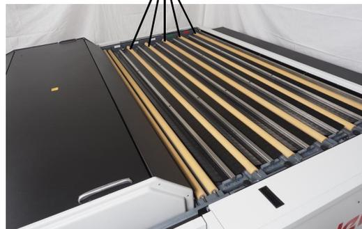
Water rinsed cross over rollers are in place in order to minimize the chemical carry over from one tank to the next as well to keep the cross over section clean and free from any chemical deposits.
