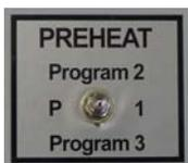
← In addition, a 3 position switch is provided for selecting the required pre-heat temperature in accordance with the plate-thickness being used. (0.15, 0.20 or 0.30mm - each thickness requires a different pre-heat temperature level). The temperature of each pre-heat setting is pre-programmable.
