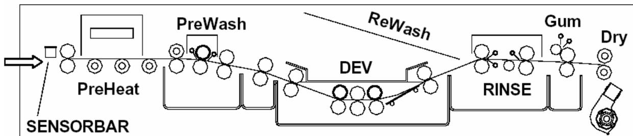
PreHeat section → PreWash section → Developer section → Rinse section → Gum section → Dry section
