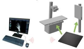
2 Flat Panel Detectors are used with only one console by our COLENTA DX Easy Imaging Software.
