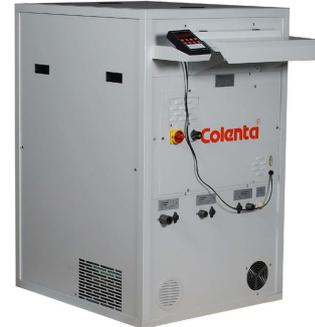
The **Colenta MP903**, as all Colenta medical X-Ray processor models, provides a fully automatic „dry to dry“ film processing technology. A microprocessor system ensures precise temperature control of all processing chemistries with automatic Developer / Fixer tank cooling to prevent overheating. Replenishment is preheated by injection into the inline chemical heating systems, which are controlled to pre-set programmed temperatures within +/- 0,2 °C.
