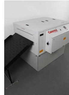
The NG Processor is available in **56, 66, 80, 95 and 110cm process widths.**
