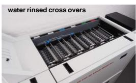
Transport rack assemblies can be manually handled into and out of the processer tanks, a rack carrier/drip tray is provided to transfer each rack from the processor to a washing area for cleaning.
