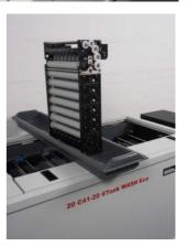
All top coves are designed for easy removal for carrying out shut-down and start-up cleaning procedures – an evaporation cover prevents any risk of contamination.
