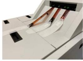
3 tracks of 135 camera film on a 20cm Filmprocessor, attached to the film leader and loaded via the multi track loading guide. The same system can be used for 120/220 film format.
