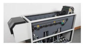
All Colenta Film processors support a maintenaince free and reliable chain drive system to drive the wet racks and dryer module.
